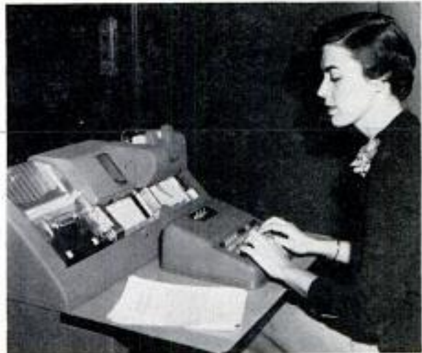
Sentences in Russian are punched on standard IBM cards for feeding into processor for translation
